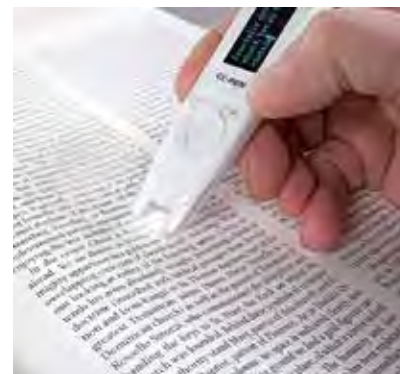
C-Pen readers are state-of-the-art devices that can scan and read words aloud in a natural voice. They can also define words, and do not require an internet connection.
