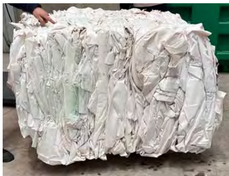
Baled building shrink wrap.
