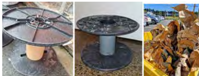
Figure 3: Left: Cable reel made of plastic, cardboard and metal fasteners. Centre: Cable reel made of #5 PP and a #3 PVC core. Right: Material cover made of plastic and paper.
