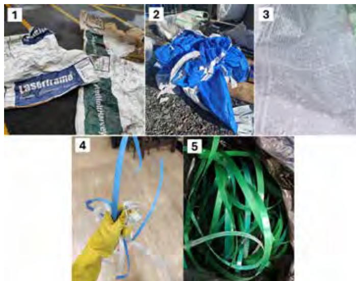
Figure 5: 1: Woven PP timber covers. 2: Woven LDPE sheets. 3: Woven LDPE Clear sheets. 4: PP strapping — woven, tangled and with metal buckles. 5: PET strapping.
