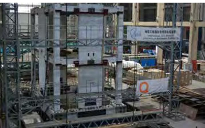
Full-scale shake-table test of a low-damage concrete wall building at Tongji University.
